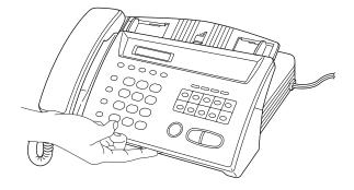
**2** Pull up the blue release lever so you can remove the three protective sheets (initial set up) or any paper remaining in the machine from the last roll.
